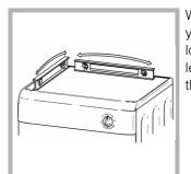
When you have installed your dryer in its final location check that it is level first side to side, then front to back.
